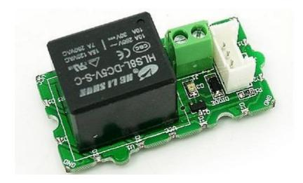
The relay Grove is a digital normally-open switch that controls a relay capable of switching much higher voltages and currents than your normal Seeeduino boards. When set to HIGH the LED will light, and the relay will close allowing current to flow. The peak voltage capability is 250V at 10 amps.
