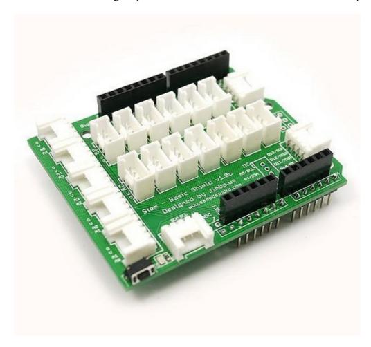
The purpose of the Grove - base shield is to allow easy connection of any microprocessor input and output pins to the small units. Each socket is clearly labelled with its matching I/O pin. For a more detailed examination of the Base Shield, please consider the following diagram:
