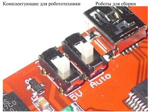
This ensures the board is running at 5V DC from the USB cable, and that the board will auto-reset upon uploading your sketch. Otherwise you will have to manually reset your <u>Seeeduino</u> before the sketch starts operation.
