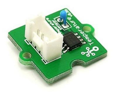
The temperature sensor Grove uses a <u>thermistor</u> which returns the ambient temperature in the form of a resistance value, which is then used to alter Vcc (5V with our Seeduinos). Our board then converts this voltage value measured by an analog input pin to a temperature. The operating range is -40 to 125 degrees Celsius, with an accuracy of  $\pm 1.5$ °C.
