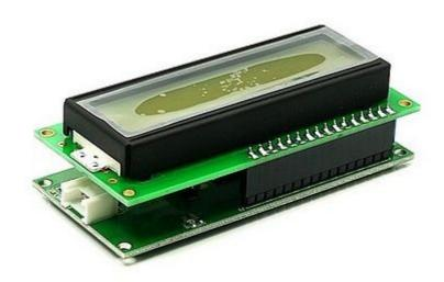
This consists of two parts, a module holding an 16 character by 2 line LCD, and the Grove itself(most may receive the two-units-soldered together-version). The LCD has an interface that is easily used under the Arduino <u>IDE</u> using the special <u>Seeedstudio SerialLCD library</u>.
