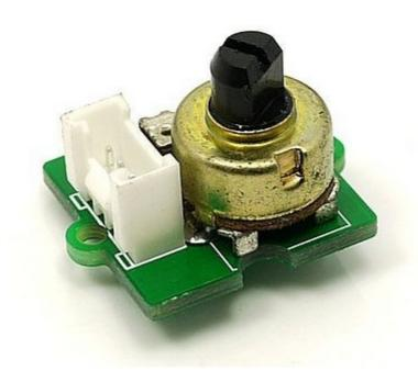
The potentiometer Grove produces analog output between 0 and Vcc (5V DC with Seeeduino) on its D1 connector. The D2 connector is not used. The angular range is 300 degrees with a linear change in value. The resistance value is 10k ohms, perfect for Arduino use. This may also be known as a "rotary angle sensor".
