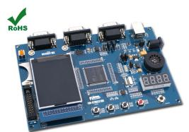
This is the low cost development kit for STM32F103ZE (72MHz, the very popular ARM Cortex-M3 processor), including the STM32F103ZE evaluation board (STM3210E Board) (SZE1) and Emlink for ARM(EAH1) JTAG adapter, so the developers can easy start to learn and test all the relevant applications on it, or evaluate your new project design through this entire system.
