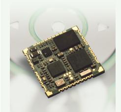
The eMD3620F ezRide-22 module is housed in a 22.0 x 22.0 x 3.0 mm SMD package that includes all the required components for a complete GPS/AGPS solution.
