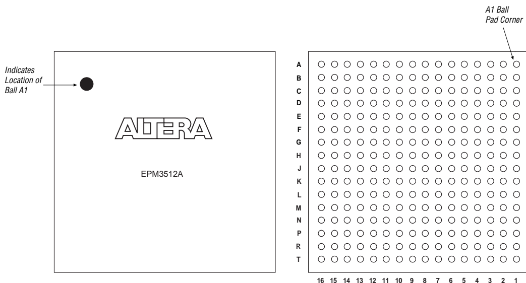
Figure 18. 256-Pin FineLine BGA Package Pin-Out Diagram
