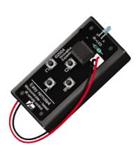
The Easy remote4 (ER-4) is a multi-purpose infrared remote control which sends out analog data mixed into the 38kHz carrier frequency.
