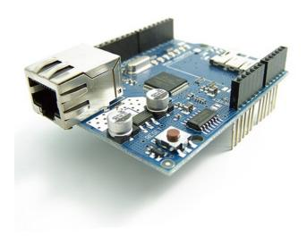
To use the shield, mount it on top of an Arduino board (e.g. the Diecimila). To upload sketches to the board, connect it to your computer with a USB cable as you normally would. Once the sketch has been uploaded, you can disconnect the board from your computer and power it with an external power supply.
