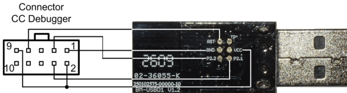
Figure 3-15. eZ430-Chronos RF Access Point Connection to CC Debugger
