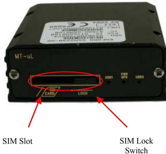
**Figure 10 – SIM Slot and SIM Lock**
