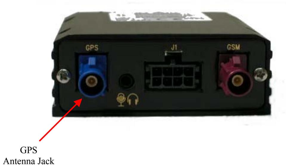
**Figure 9 – GPS Antenna**
