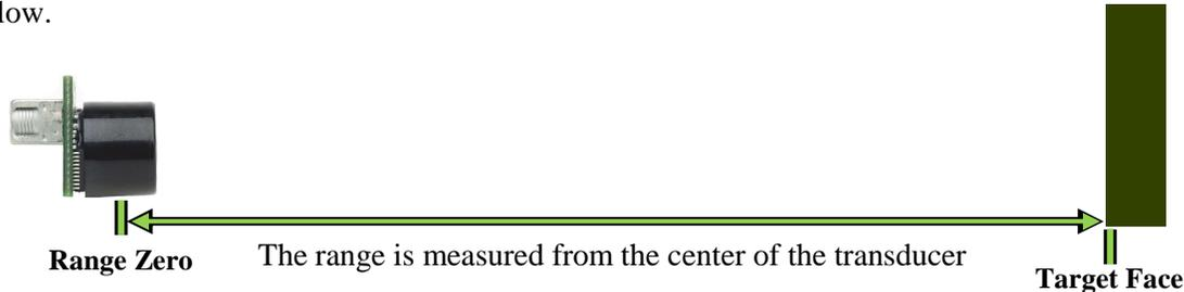
The I2CXL-MaxSonar-EZ will report the range to the closest detectable object. Target detection has been characterized in the sensor beam patterns.
