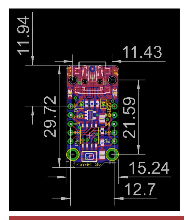
There are <code>[two]</code> versions of the Trinket: 3V and 5V. They are almost identical but there are slight differences in the pinouts: one has a 3V output pin in the bottom right, the other has a 5V output pin instead
