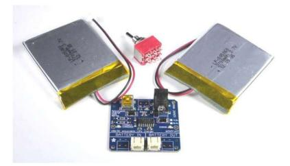
Lithium Polymer Batteries pack a lot of power in a small package. But they can be tricky to charge safely. The Adafruit LiPo Chargers all provide a charging cycle designed to safely charge 3.7v Lithium Polymer cells. But what if your project needs more than 3.7v?
