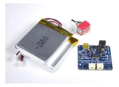
This charger assures that the cells are 'balanced' at all times by charging them in parallel. When the cells are connected in parallel, any difference in charge level is equalized and they appear as a single cell to the charger. At all times during the charge, the cells are at equal charge levels.
