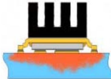
② Mounted to a PCB with small clip heatsink (still air)
