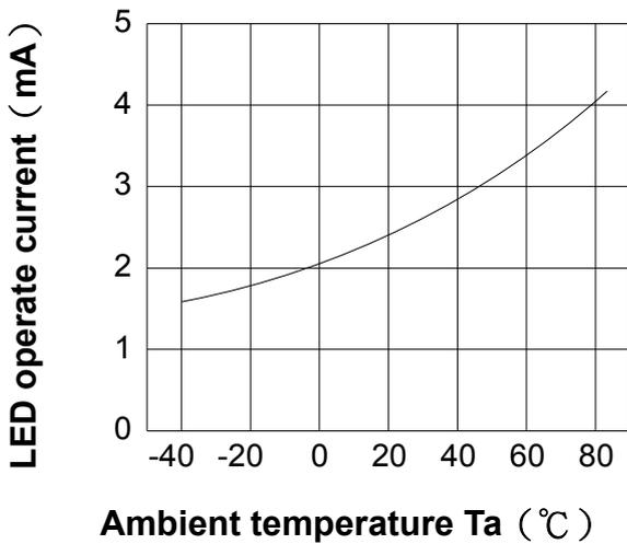
**LED Reverse ( ON ) current vs. ambient temperature**
