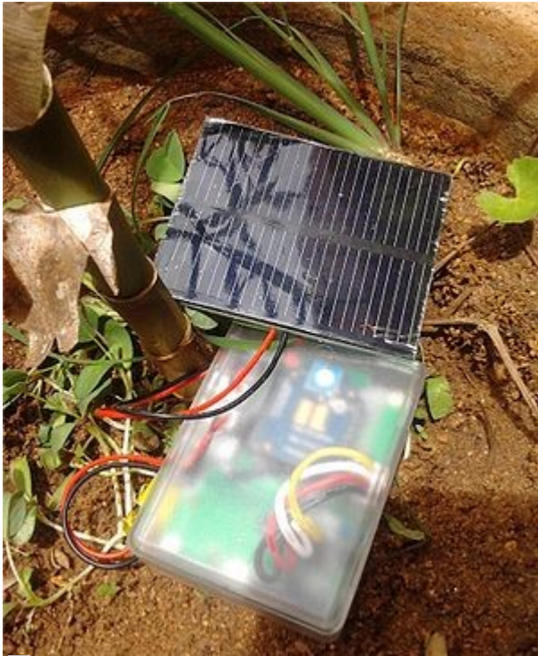
Wireless Sensor Node Field Use - Charged by Solar Panel"
