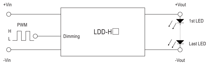
Fig-1 12VDC input, 1~3 LEDs (Vf=3V)
