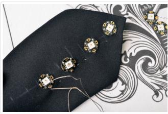
Add a few more pixels by connecting this long ground line to the (-) pads on the pixels.
