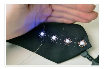
Stitch up the rest of the pixels - you'll have one long ground bus, one long power bus, and short segments between each input/output data pads.
