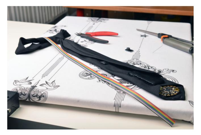
Cut a piece of ribbon cable longer than the main part of the tie.
