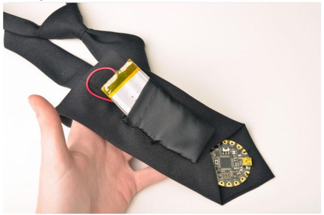
Use a piece of scrap fabric to stitch a small pouch for your lipoly battery. The pouch should be stitched to the back of the tie, just above where the Flora goes, and have an opening at the top for easy removal of the battery for charging. Use a seam ripper to open up the back seam of the tie just a little so you can thread the JST plug and wire inside the tie and down to the Flora.
