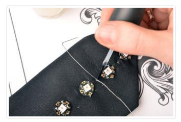
Use another long length of conductive thread to connect Flora's VBATT pad to the (+) pads on the pixels.
