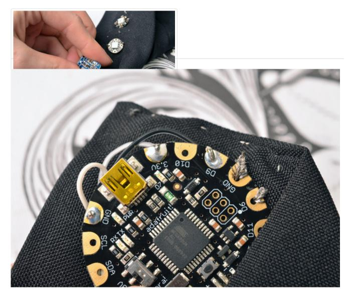
Back at the Flora end of the board, solder the corresponding wires to 3.3V, GND, and D9.
