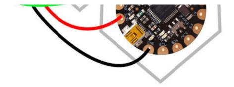
The Flora pixels are all connected to common ground bus, as well as a common power bus connected to VBATT. The Flora pixel data bus is connected to D6. The microphone amplifier is connected to 3.3V, GND, and D9.
