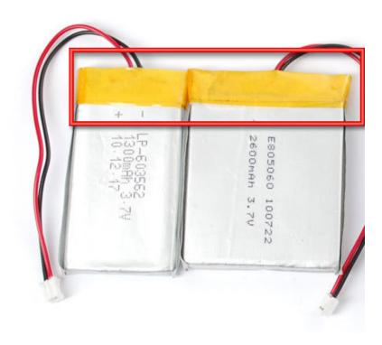
If you don't see any taped circuit board, the cell may be 'raw' - these raw cells **are not** protected!
