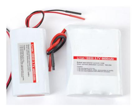
The answer is that these batteries are assembled by a company that is experienced and certified to test and assemble battery packs. The individual batteries are tested and sorted by machine so that each pack has matching batteries with the same capacity and internal resistance. Individuals do not have this equipment, which is why you should not try to make your own packs.
