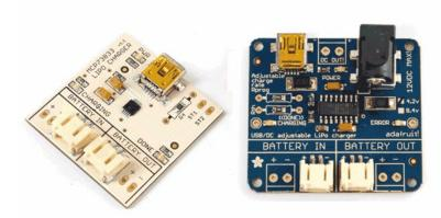
We carry two chargers in our store (at this time). A USB charger and a USB/DC charger. The USB charger is meant for charging single cells from a USB port that can provide 500mA or so. The USB/DC charger is meant for charging batteries from a USB port **or** a DC power supply up to 12V. The latter is more flexible, but more expensive because of the added circuitry.
