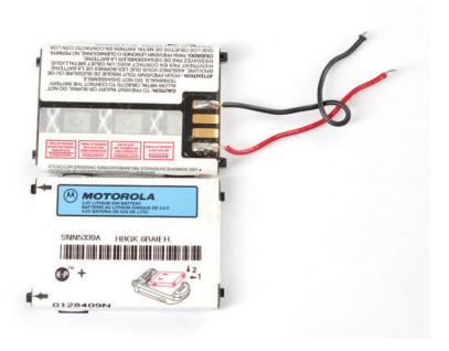
You may end up using camcorder or cell phone batteries. These are removable batteries in a hard case. They tend have protection cells inside the case. This battery for example, is an old project battery from before you could buy lipoly batteries easily.
