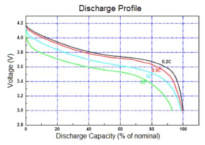
Discharge: 3.0V cutoff at room temperature.
