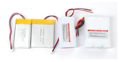
On the left you can see two Lithium Ion Polymer cells. On the right, two packs made of cylindrical Lithium Ion batteries
