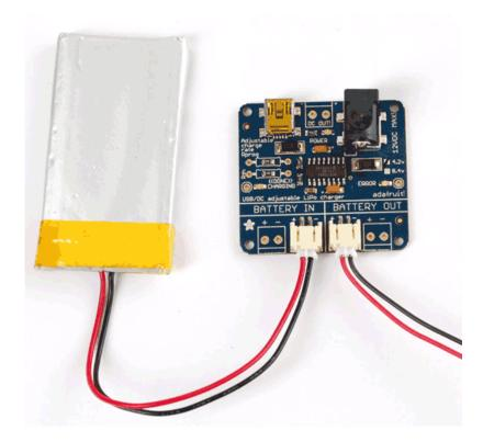
If you want to use the battery while also having it connected to the charger (less plugging and unplugging that way) you can simply use the **BATTERY OUT** connection on the right. The **IN** and **OUT** ports are connected together on the circuit board so it acts as a *pass-through*
