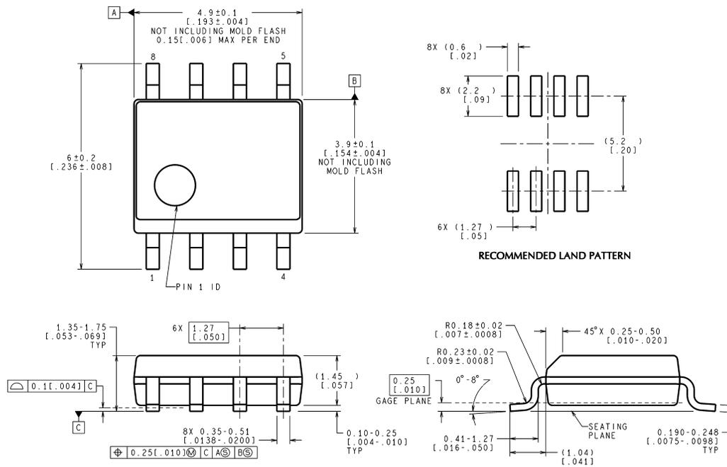
CONTROLLING DIMENSION IS MILLIMETER
