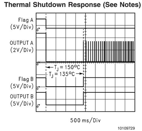
\* Port A is shorted to GND through a 100 mΩ resistor
