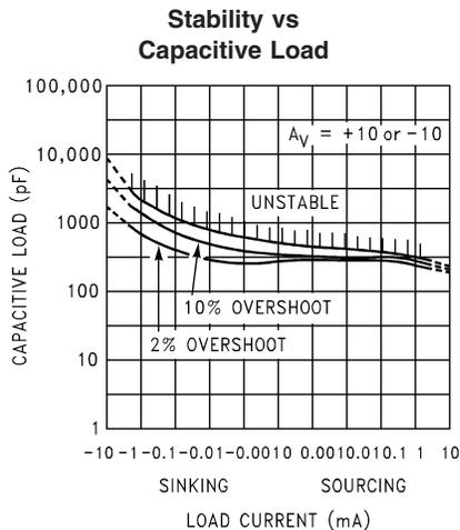
**Note 13:** Avoid resistive loads of less than  $500\Omega$ , as they may cause instability.
