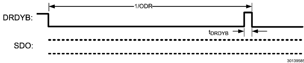
FIGURE 21. DRDYB Behavior for an ADC_DOUT not Read
