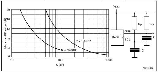
Figure 4. Maximum R<sub>P</sub> Value versus Bus Parasitic Capacitance (C) for an I<sup>2</sup>C Bus
