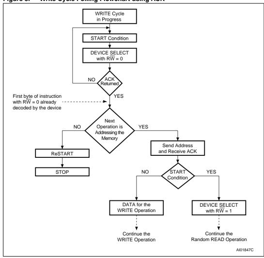
Figure 8. Write Cycle Polling Flowchart using ACK
