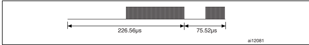
Figure 38. Start of frame, low data rate, one subcarrier x2
