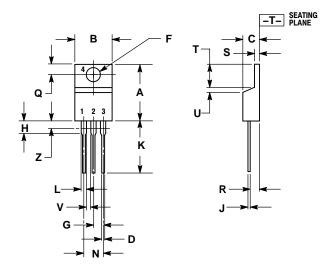
NOTES: 1. DIMENSIONING AND TOLERANCING PER ANSI Y14.5M, 1982. CONTROLLING DIMENSION: INCH.
