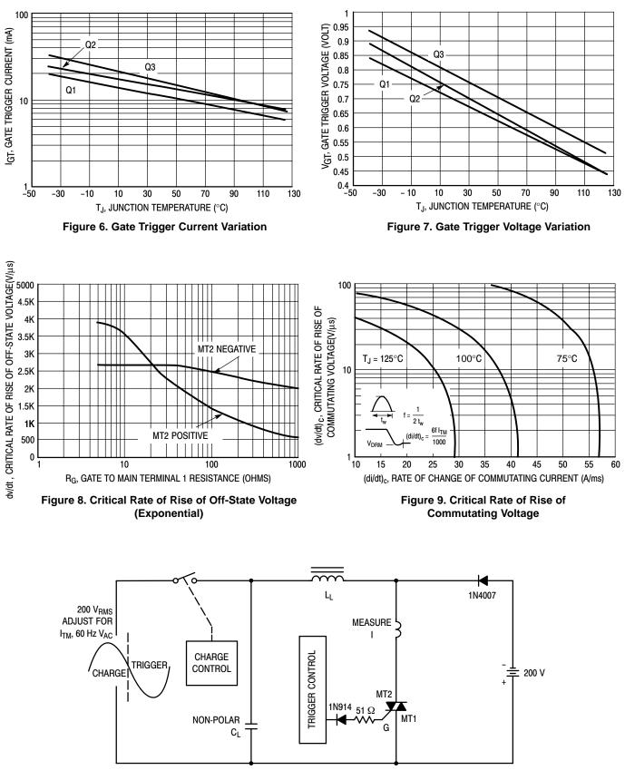
Note: Component values are for verification of rated (di/dt)<sub>c</sub>. See AN1048 for additional information.
