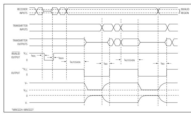
Figure 4b. AutoShutdown Plus, INVALID, and READY Timing Diagram
