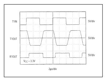
Figure 9. MAX3224/MAX3226/MAX3244 Loopback Test Result at 250kbps
