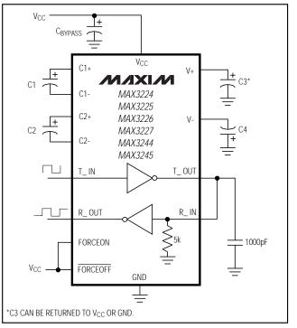
Figure 7. Loopback Test Circuit
