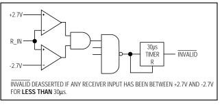
Figure 3b. INVALID Functional Diagram, INVALID High
