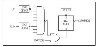
Figure 3c. AutoShutdown Plus Logic
