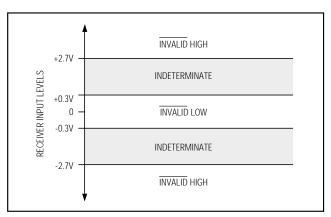
Figure 4a. Receiver Positive/Negative Thresholds for INVALID
