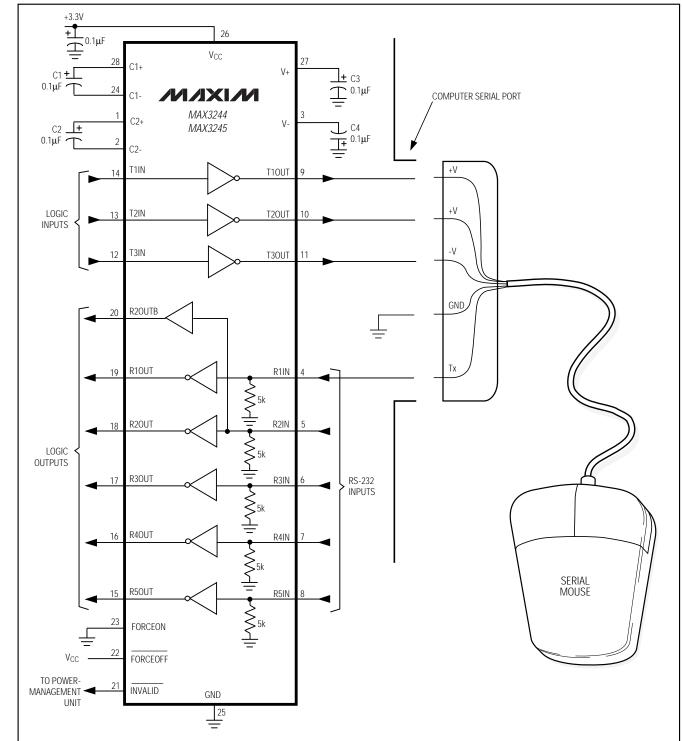
Figure 11b. Mouse Driver Test Circuit
