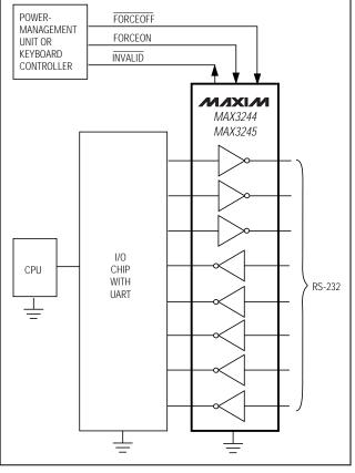
Figure 1. Interface Under Control of PMU
