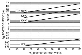
Figure 2. Typical Reverse Current\*
