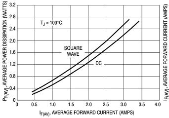
Figure 3. Power Dissipation
