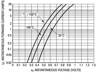
Figure 1. Typical Forward Voltage
