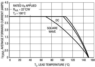
Figure 4. Current Derating, Lead
