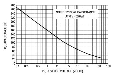
Figure 5. Typical Capacitance
