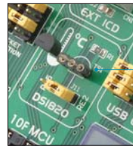
Figure 10-4: DS1820 plugged into appropriate socket
