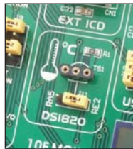
Figure 10-3: J11 in the right-hand position (1-wire communication through the RE2 pin)
