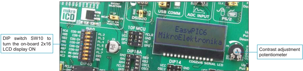
Figure 16-1: On-board 2x16 LCD display
