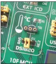
Figure 10-1: DS1820 connector (1-wire communication is not used)
