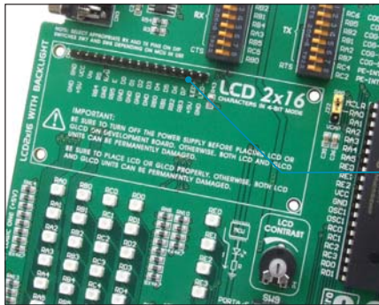
Figure 15-1: Alphanumeric LCD connector
