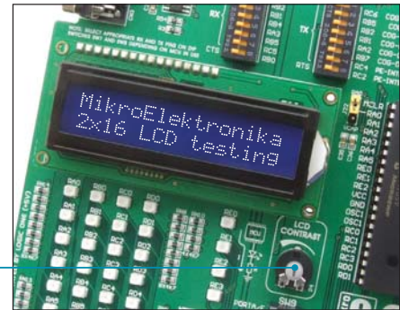
Figure 15-2: 2x16 LCD display
