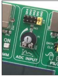
Figure 11-2: The RA0 pin used as A/D conversion input
