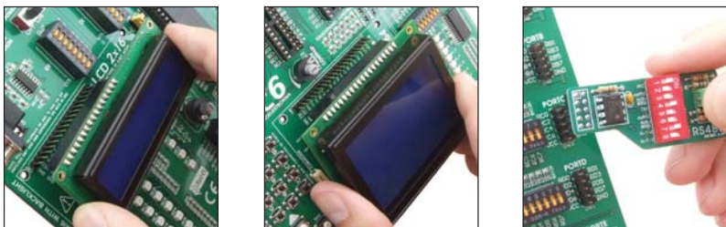
Figure 1-3: Placing additional modules on the board
