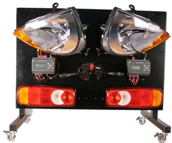
Automotive training panel running with two CAN connected MIAC devices.
