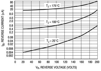
Figure 2. Typical Reverse Current\*
