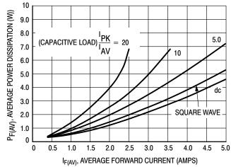
Figure 3. Power Dissipation
