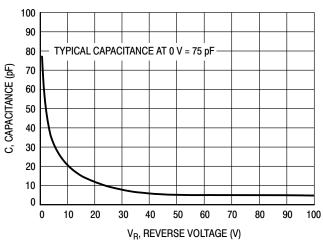
Figure 10. Typical Capacitance
