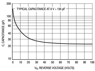
Figure 5. Typical Capacitance
