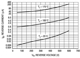
Figure 7. Typical Reverse Current\*
