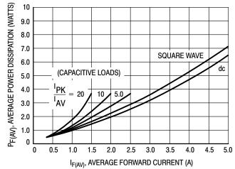
Figure 8. Power Dissipation
