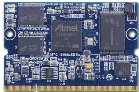
Figure 1-5 MYC-SAMA5D3X CPU Module Controller Board of MYD-SAMA5D3X
