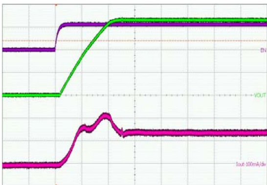
( V_{IN} = 5\text{ V} , I_{LOAD} = 100\text{ mA} , L = 3.3\text{ }\mu\text{H} , C_{OUT} = 2 \times 22\text{ }\mu\text{F} ) Upper Trace: EN Pin Voltage, 2 V/div Middle Trace: Output Voltage, 1 V/div Lower Trace: Inductor Current, 100 mA/div Time Scale: 500 \mu\text{s/div}
