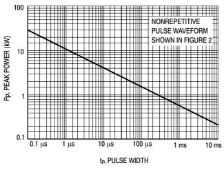
Figure 1. Pulse Rating Curve
