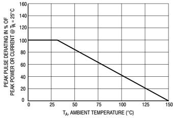
Figure 3. Pulse Derating Curve
