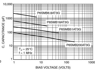
Figure 4. Typical Junction Capacitance vs.
