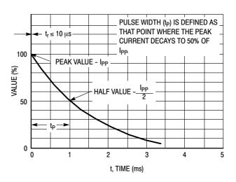
Figure 2. Pulse Waveform
