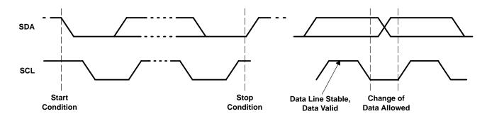
Figure 3–10. Serial Bus Start/Stop Conditions and Bit Transfers
