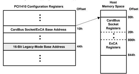
Figure 5–2. ExCA Register Access Through Memory
