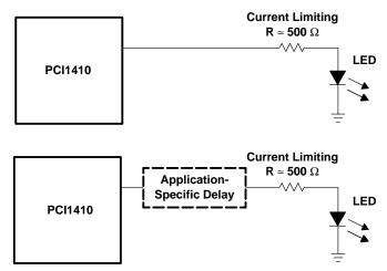
Figure 3–8. Two Sample LED Circuits
