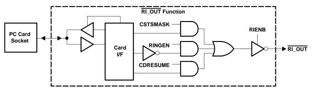
Figure 3–19. RI\_OUT Functional Diagram
