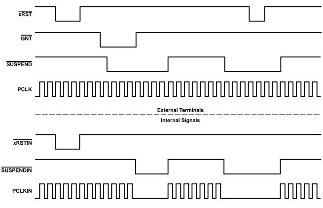
Figure 3–18. Signal Diagram of Suspend Function
