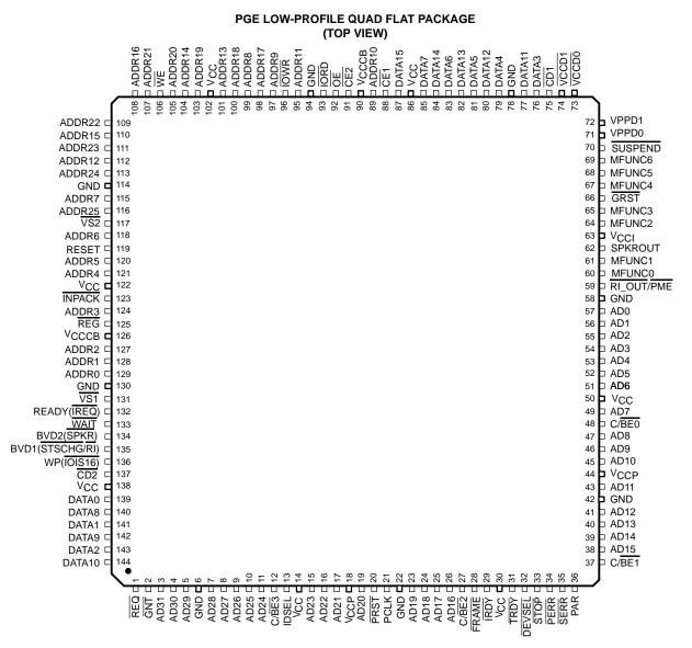
Figure 2–2. PCI-to-PC Card (16-Bit) Terminal Diagram
