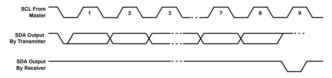
Figure 3–11. Serial Bus Protocol Acknowledge
