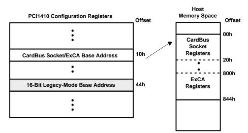
Figure 6–1. Accessing CardBus Socket Registers Through PCI Memory
