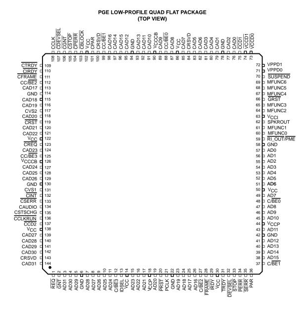
Figure 2–1. PCI-to-CardBus Terminal Diagram
