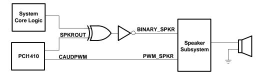
Figure 3–7. Sample Application of SPKROUT and CAUDPWM
