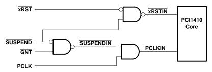
Figure 3–17. Suspend Logic Diagram
