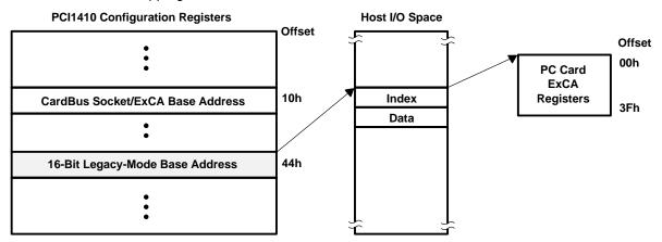
Figure 5–1. ExCA Register Access Through I/O
