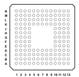
Figure 2–3. GGU Package Terminal Diagram
