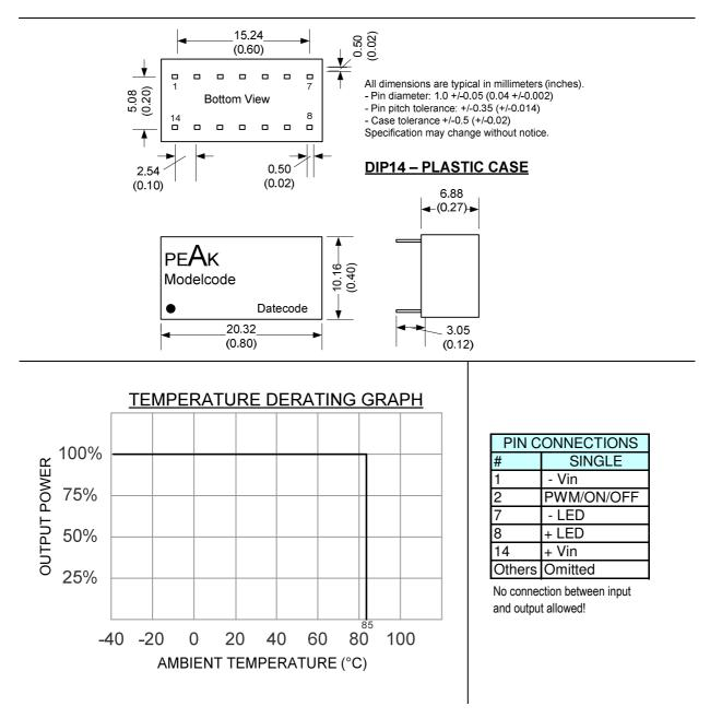
PMLEDS-Series – PLED-S-xxxLF – Single Output – DIP14 - Plastic Case Specification can change without a notice – We accept no liability for any inaccuracy or printing errors. Page 2/6
