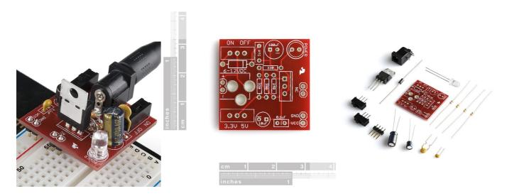
**Description:** A very simple breadboard power supply kit that takes power from a DC wall wart and outputs a selectable 5V or 3.3V regulated voltage. The .1" headers are mounted on the bottom of the PCB for simple insertion into a breadboard. Pins labeled VCC and GND plug directly into the power lines. The lone pair of pins have no electrical connection but help support the PCB.
