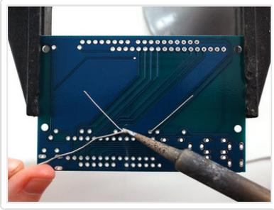
With your soldering iron heated up and ready, solder in both leads of the resistor. To do this, heat up the round ring pad and the wire lead at the same time for 2 or 3 seconds, then dip the end of the solder into the heated joint to melt it in.
