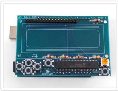
Next, check if you have an RGB LCD (with 18 pins) or a Monochrome display (not RGB, with 16 pins).
