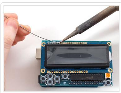
Solder all the pins to the LCD display.
