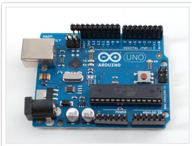
Place the header onto your Arduino, if you have an R2 or earlier arduino, there will be two pins that 'hang over' past the AREF breakout. These two extra pins are used for R3 and later Arduino classics and Mega's to make connecting to the I2C pins easier. We suggest keeping those two pins in case you ever upgrade your 'duino.
