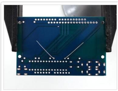
Bend the 'legs' of the resistor out so it sits flat against the PCB and flip it over.
