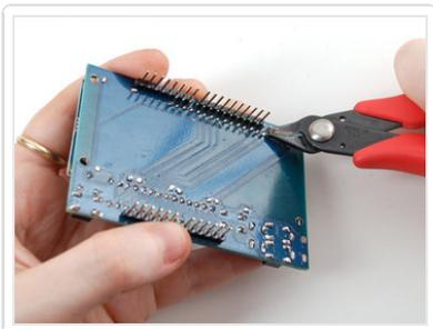
Finish up by carefully clipping the leads. For some Arduinos, the long leads may interfere with headers or parts on the Arduino board so we suggest just clipping them all. Do it carefully as these are a little difficult to cut and may fly at you. We suggest doing it over a trash can.
