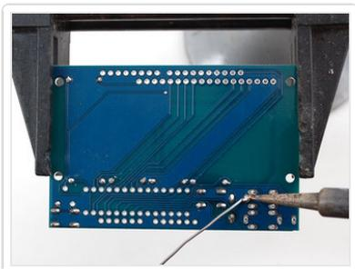
Solder each leg, taking care not to accidentally 'short' two button legs together. The ones for the directional pads are very close!
