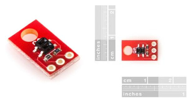
**Description:** This version of the QRE1113 breakout board features an easy-to-use analog output, which will vary depending on the amount of IR light reflected back to the sensor. This tiny board is perfect for line sensing applications and can be used in both 3.3V and 5V systems.
