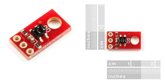
**Description:** This version of the QRE1113 breakout board features a digital output, using a capacitor discharge circuit to measure the amount of reflection. This tiny board is perfect for line sensing when only digital I/O is available, and can be used in both 3.3V and 5V systems.
