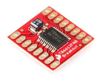
**Description:** The TB6612FNG motor driver can control up to two DC motors at a constant current of 1.2A (3.2A peak). Two input signals (IN1 and IN2) can be used to control the motor in one of four function modes - CW, CCW, short-brake, and stop. The two motor outputs (A and B) can be separately controlled, the speed of each motor is controlled via a PWM input signal with a frequency up to 100kHz. The STBY pin should be pulled high to take the motor out of standby mode.
