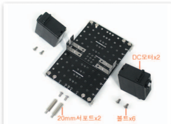
3 Fix the DC Motors to the Motor Frames with bolts and then fix the 20mm Support to the Main Frame with bolts.
