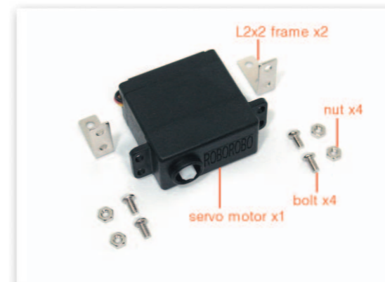
5 Fix the Servo Motor and the L-type 2x2 Frame with bolts and nuts.
