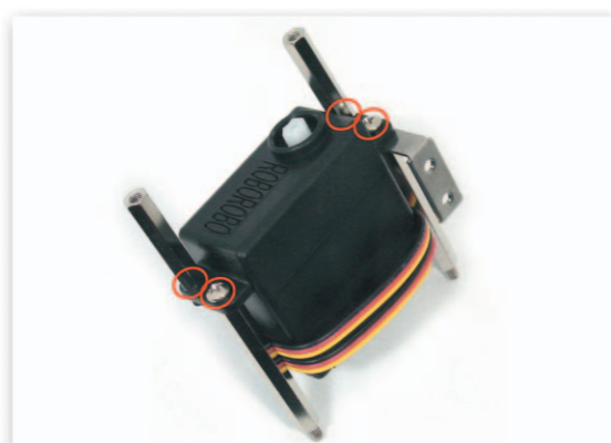
9 Overlap the 25mm Supports and the 40mm Supports to the Servo Motor on the Motor Frame and fix with bolts and a nut.
