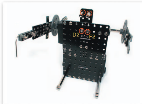
13 Fix the 20mm Supports to the Option Frame and then fix to the Main Frame with bolts and nuts.
