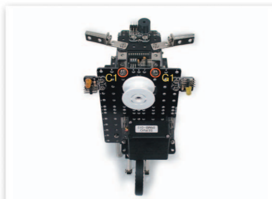
20 Fix the L-type 2x2 Frame of the Handle part to the Main Frame with bolts and nuts.
