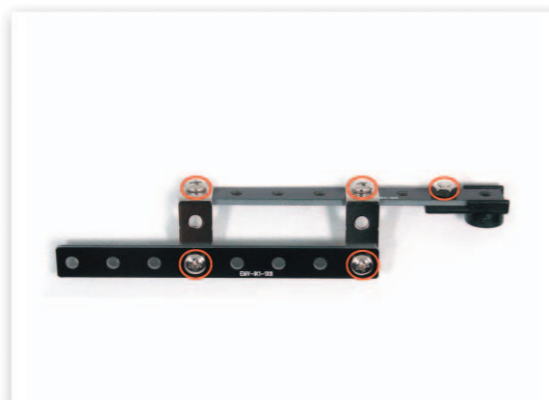
13 Connect 2 the two Small 8 Frames with the L-type 2x1 Frame and then fix the Motor Guide to the Small 8 Frame.
