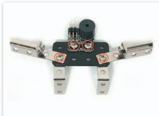
19 Fix the Buzzer Board to the Option Frame and then put Option Frame in the middle, overlap the L-type 2x1 Frame and the L-type 2x2 Frame up and down and fix with bolts and nuts to make handle parts.
