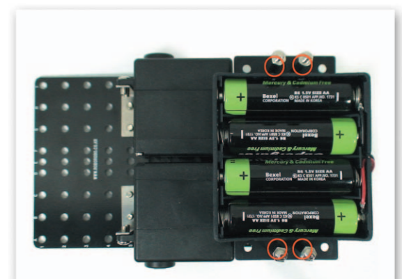
5 Insert the Battery Case to the Support that is fixed to the Main Frame and fix with the 20mm Support.
