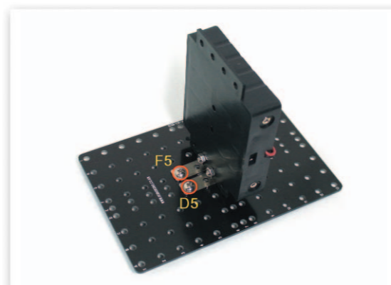
2 Fix the L-type 2x1 Frame that is fixed to the Battery Case to the Main Frame.
