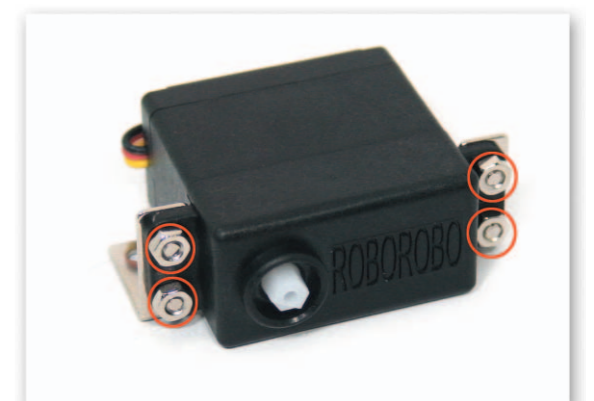
5 Fix the Servo Motor and the L-type 2x2 Frame with bolts and nuts.
