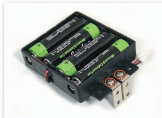
1 Fix the L-type 2x1 Frame on the Battery Case with bolts and nuts.
