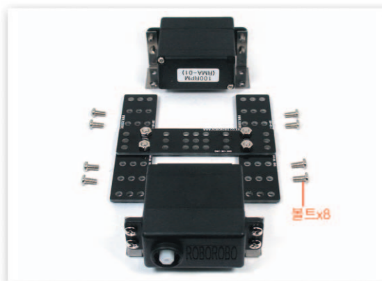
3 Put the Motor Frame that is fixed to the DC Motor on the Middle Frame and fix only with bolts.
