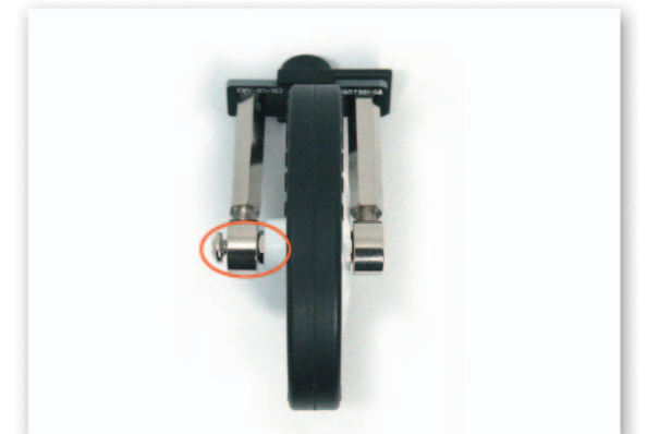
16 Insert the 7mm Support that is fixed to the Wheel first and then fix the regulable bolt on the other side with the 3x10 Bolt.
