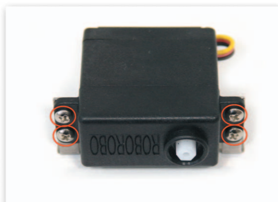
2 Fix the Motor Frame that is fixed to the DC Motor to the Main Frame with bolts.
