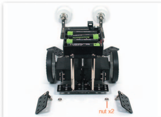
14 Put the Support that is fixed to the Option Frame on the Middle Frame and fix with nuts.
