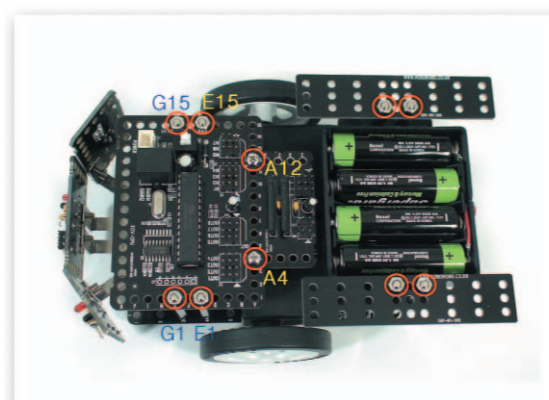
9 Connect the CPU Board and the DC Motor Drive Board with bolts and nuts then insert it to the Support that is fixed to the Main Frame with nuts. Insert the Middle Frame to the Support that is fixed to the Battery Case and fix with nuts.
