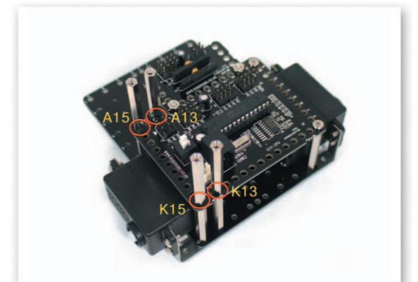
4 Connect the 35mm Support to the Support that holds the CPU Board.
