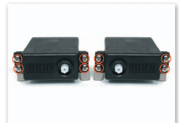
5 Fix the DC Motor and the Motor Frame using only bolts.
