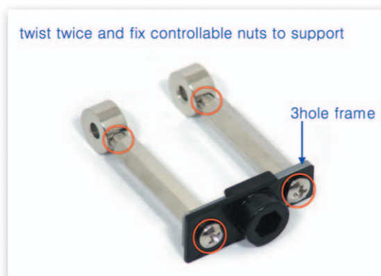
15 Insert bolts after overlapping the Motor Guide and the Small 3 Frame and then fix with the 25mm Support. Also twist about twice and fix the regulable bolt to the 25mm Support.
