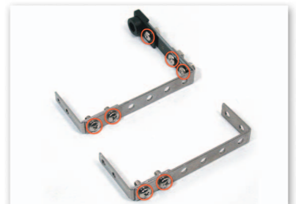
10 Connect the Motor Frames and the L-type 2x6 Frames with bolts. Then overlap the Small 5 Frame and the Motor Guide on the L-type 2x6 Frame and fix with bolts and nuts.
