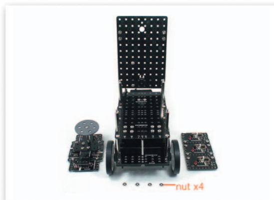
14 Put the Contact Sensor Board and the Infrared Sensor Board on the Support that is fixed to the Main Frame and fix with nuts.
