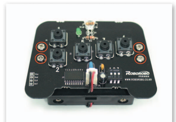
18 Fix the 7mm Support to the Battery Case and then put the Remote Control Sending Board on it and fix with bolts. Completed Wireless Remote Control.
