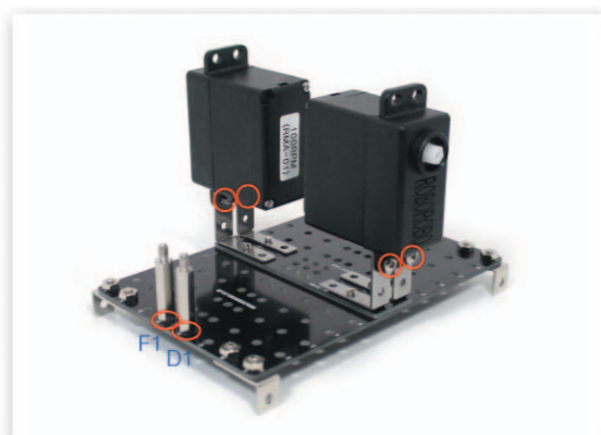
3 Fix the DC Motors to the Motor Frames with bolts and then fix the 20mm Support to the Main Frame with bolts.
