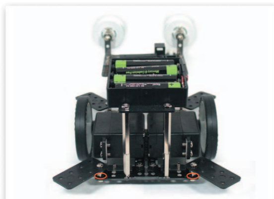
14 Put the Support that is fixed to the Option Frame on the Middle Frame and fix with nuts.
