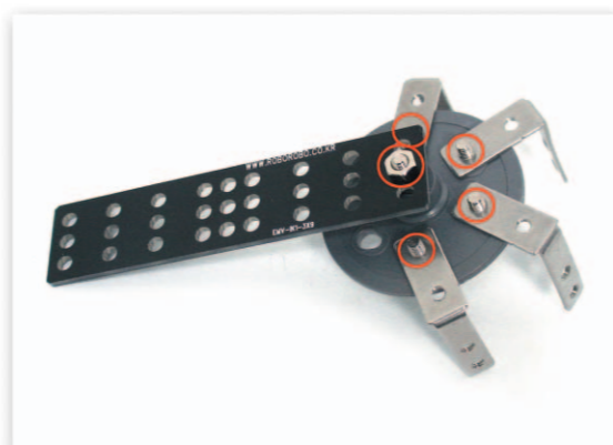
14 Fix the Motor Frame to the Wheel Guide with bolts then fix the Wheel Guide and the Middle Frame with a nut.
