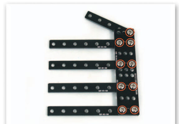
12 Fix the Small 8 Frame and the Small 5 Frame to the Middle Frame with bolts and nuts and make a shape of a hand.
