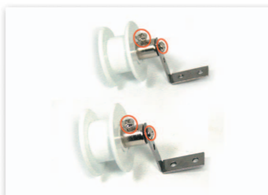
9 Fix the 3x10 Bolts to the Motor Frame then insert the Caterpillar Wheel Guide to the 3x10 Bolts and fix with bolts.
