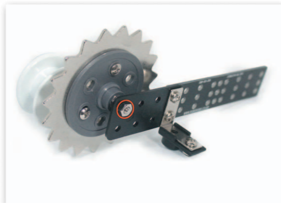
13 Fix the Support that is fixed to the Wheel Guide to the Option Frame with a nut.
