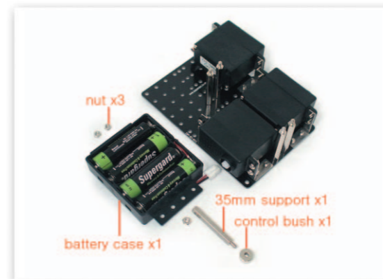
6 Put the Battery Case to the Support that is fixed to the Main Frame and fix with nuts and 35mm Support. Then fix the regulable nut to the 35mm Support.
