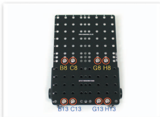
2 Fix the Motor Frame that is fixed to the DC Motor to the Main Frame with bolts.
