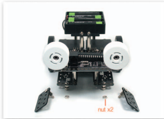
13 Put the Support that is fixed to the Option Frame on the Infrared Sensor Board and fix with nuts.
