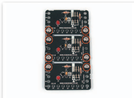
13 Put the Small 5 Frames under the Infrared Sensor Board and fix with bolts and nuts.
