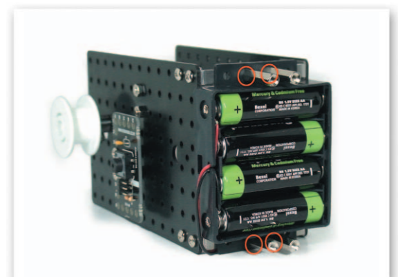
5 Put the Battery Case on the Motor Frames and fix with the 20mm Supports.
