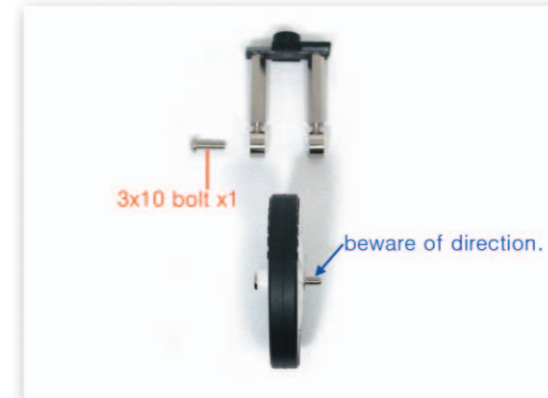
16 Insert the 7mm Support that is fixed to the Wheel first and then fix the regulable bolt on the other side with the 3x10 Bolt.
