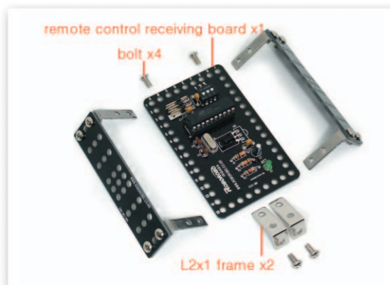
2 Fix the L-type 2x1 Frame and the Motor Frame that is connected to the Middle Frame to the Remote Control Receiving Board with bolts.
