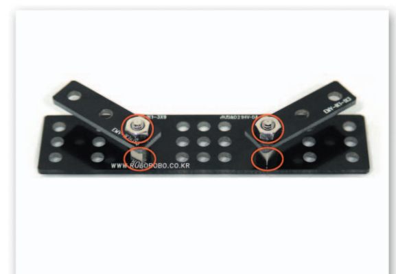
18 Fix the 7mm Support to the Middle Frame with bolts and then put the Small 3 Frame on the 7mm Support and fix with nuts.
