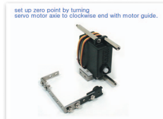
11 Insert the Motor Guide that is connected to the L-type 2x6 Frame to the Servo Motor axle.
