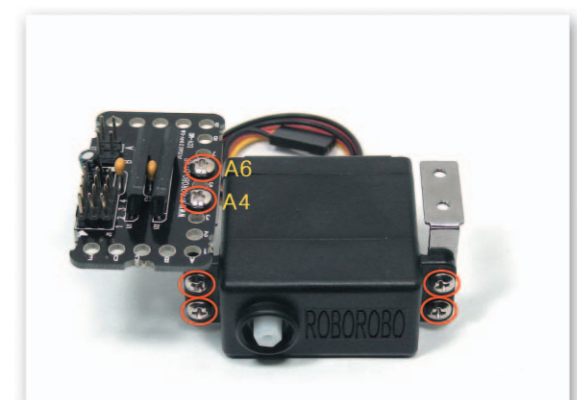
6 Fix the Servo Motor and the Motor Frames with bolts and then put the DC Motor Drive Board on the Motor Frame and fix with bolts.
