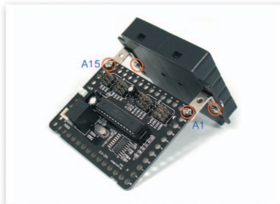
7 Connect the Battery Case and the CPU Board with the L-type 2x2 Frame.
