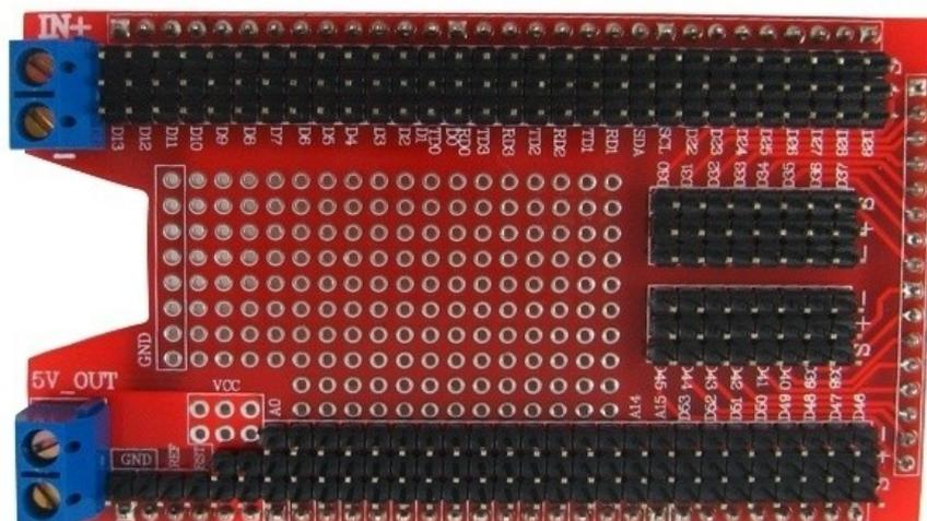
A heavy duty screw terminal allows better access to the 5V output of the 3A switch mode power supply. The PCB is smaller than the Spider so that it does not block access to the Spiders pins and reset button. This allows a mixture of low power and high power servos to be run from the Spider controller.
