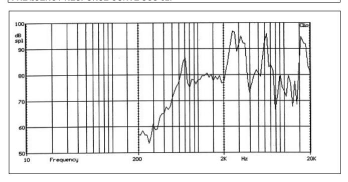
The frequency response curve is measured on an axis at a distance of 30cm at 30Vpp input voltage (sine wave) at 21° in free air. During measurement, the speaker is mounted in a closed box of 40cm H x 15cm W x 5cm. Deduct 10 dB(A) in average for use at 10Vpp.
