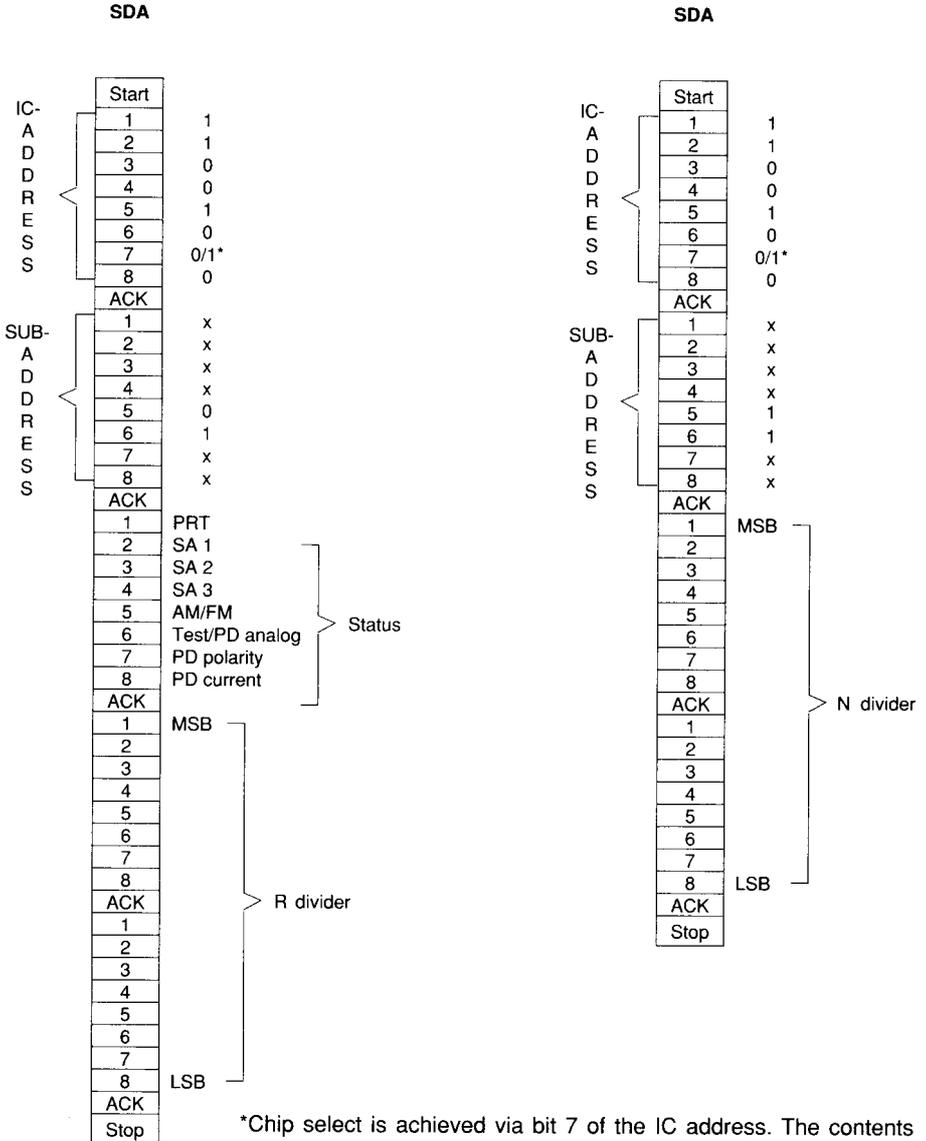
\*Chip select is achieved via bit 7 of the IC address. The contents are compared with the value set on pin A0. If the values are identical, the respective chip is selected.
