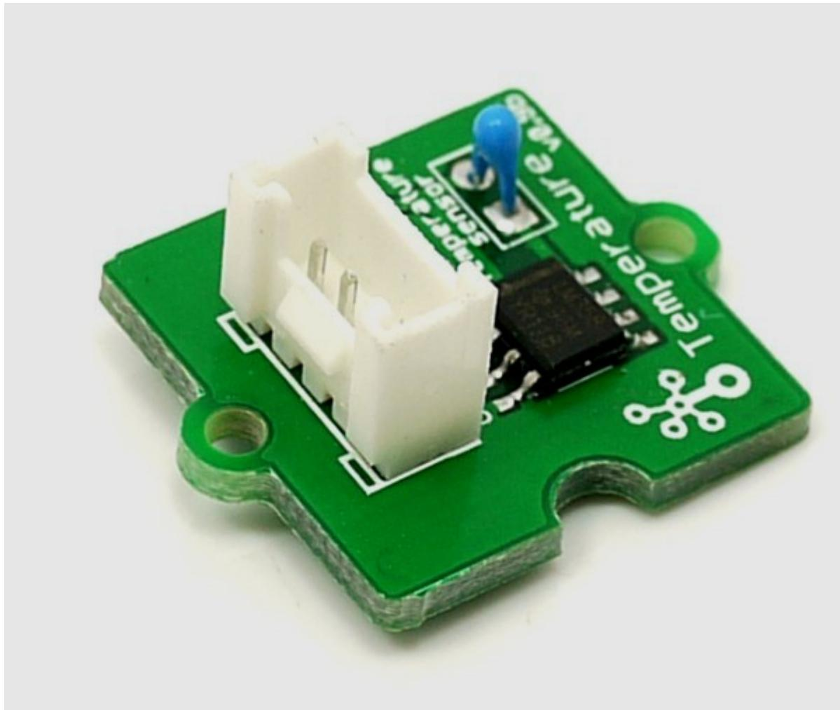
The temperature sensor Grove uses a thermistor which returns the ambient temperature in the form of a resistance value, which is then used to alter Vcc (5V with our Seeduinos). Our board then converts this voltage value measured by an analog input pin to a temperature. The operating range is -40 to 125 degrees Celsius, with an accuracy of  $\pm 1.5^{\circ}\text{C}$ .
