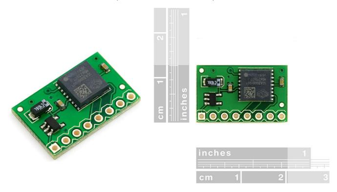
**Description:** This is a compact breakout board for the SCA3000 triple axis accelerometer from VTI. This highly precise and temperature compensated accelerometer is a good option for IMU and <u>dead-reckoning</u> applications. The low noise and temperature compensation significantly reduces drift over time.
