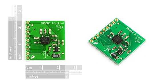
**Description:** This is the breakout board for the IDG500, which includes an on-board 2.8V regulator and all pins broken out to 0.1" pin holes. The IDG-500 is a very small, dual-axis angular rate sensor (gyroscope). It uses InvenSense's proprietary and patented MEMS technology with vertically driven, vibrating masses to make a functionally complete, low-cost, dual-axis angular rate sensor. All required electronics are integrated onto a single chip with the sensor.
