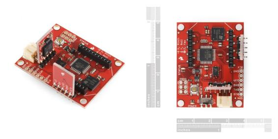
**Description:** The 6DOF Atomic is a stripped-down IMU, designed to give good performance at a low price. The unit can run as a hard-wired UART interface (0-3.3V, 115200bps), or with an XBee RF module, and is powered from a single Lithium Polymer battery. The processor is an Atmel ATMega328 running at 10MHz with 6 dedicated 10-bit ADC channels reading the sensors. Source code for the 6DOF Atomic is freely available and compiles with the free AVR GCC compiler.
