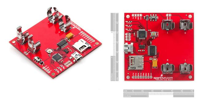
**Description:** This is an evaluation board for the ADXL345 three-axis accelerometer. The ADXL345 is an awesome little accelerometer, capable of measuring acceleration of up to  $\pm 16g$  at up to 13-bit resolution. The evaluation board includes everything you'll need to adjust the ADXL345's settings, and monitor and log its outputs.
