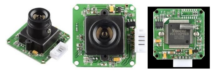
**Description:** The LinkSprite JPEG color camera allows you to capture and output JPEG images through UART, making it easy to integrate into an existing design.
