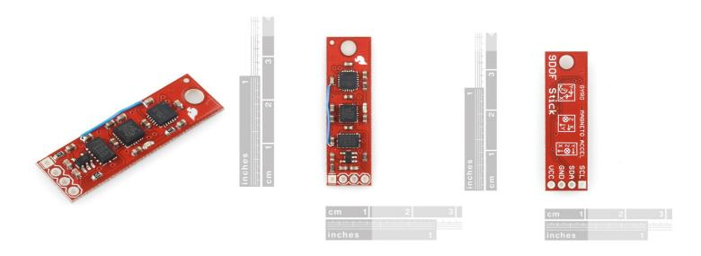
**Description:** The 9DOF Sensor stick is a very small sensor board with 9 degrees of freedom. It includes the ADXL345 accelerometer, the HMC5843 magnetometer, and the ITG-3200 gyro. The 'stick' has a simple I2C interface and a mounting hole for attaching it to your project. Also, the board is a mere 0.036" thick (0.093" overall), allowing it to be easily mounted in just about any application.
