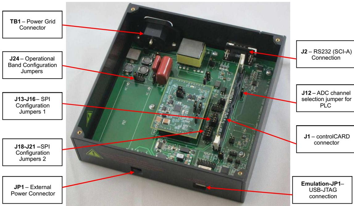
**Figure 4. TMDSPCKIT-V3 Board**
